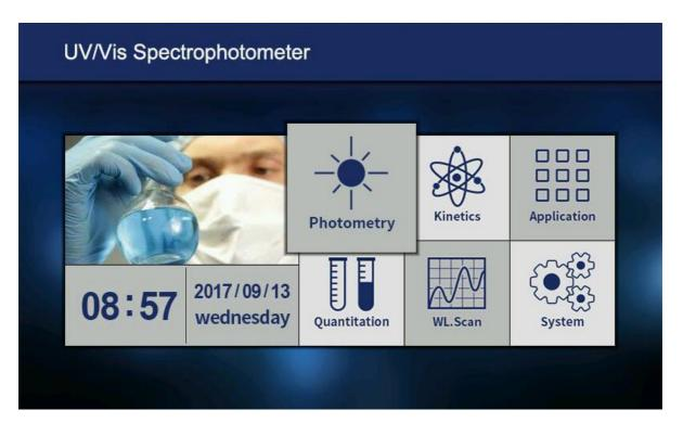
**Note:** After power on the instrument, the instrument will automatically self-test and initialization until after initialization is complete, the instrument will warm up for 20 minutes, 20 minutes warm-up time or press [ESC] to skip preheating case, the instrument being prompted preparatory work environment, which is the instrument re-calibration dark current, set the working parameters, etc., and then enter the main menu.
