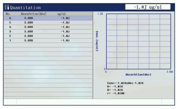
Put sample into cuvette holder and press [start] key, to get the concentration value of the current sample.
