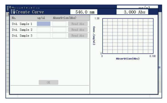
Put various standard samples into cuvette holder orderly, and enter the concentration value of each sample, then press [enter] key, read the absorbance of the sample. The input is completed, the data of the standard sample is calculated automatically according to the parameters of the curve, displayed on the screen. If the parameter is wrong, then the buzzer alarm, exit to establish the curve function.
